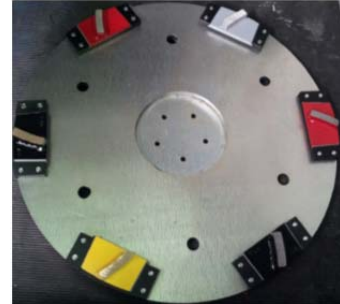
Disc with Frankfurt attachments for TMB Insert used with 3, 6 or 9 inserts of the same grain size
